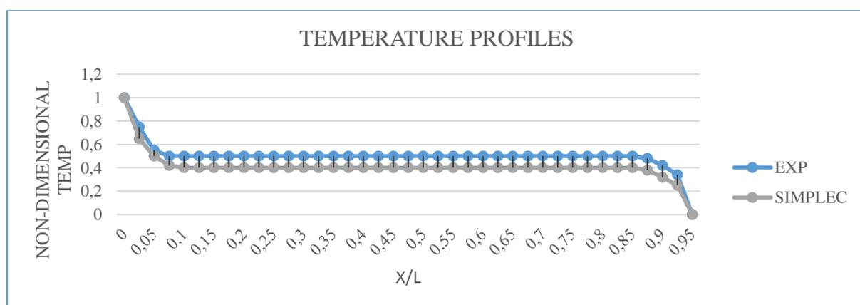
Figure 6. Comparison of the mean temperature at  $y/H=0.5$
