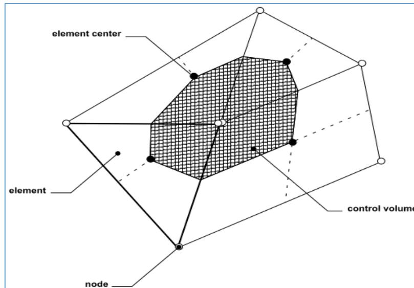
**Figure 2. Control-volume element**
