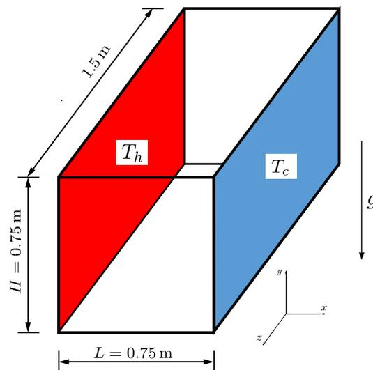
**Figure 1. Geometry of the 3-D numerical model**
