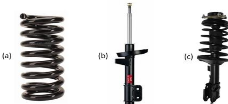
Figure 2. (a) Coil spring (b) Strut (c) Pre-assembled unit
