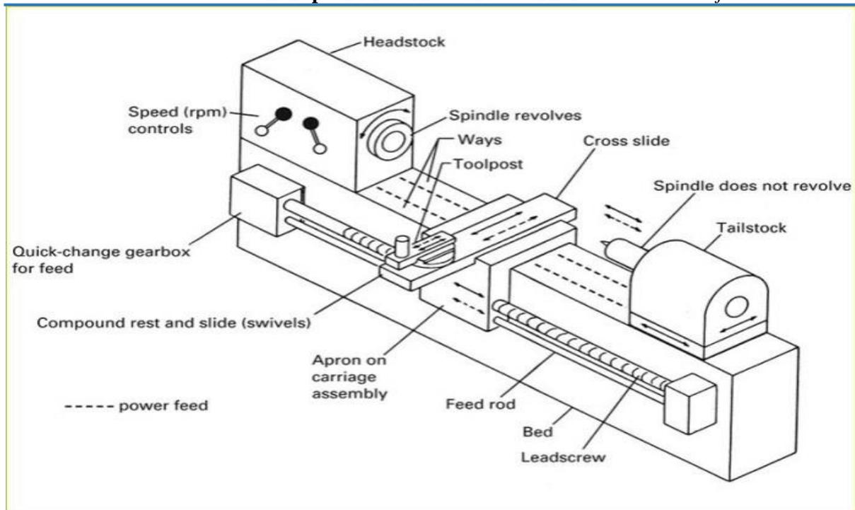
Figure 4. The principal parts of the engine lathe and movements that can be performed on it (Tuleun & Guma, 2006)
