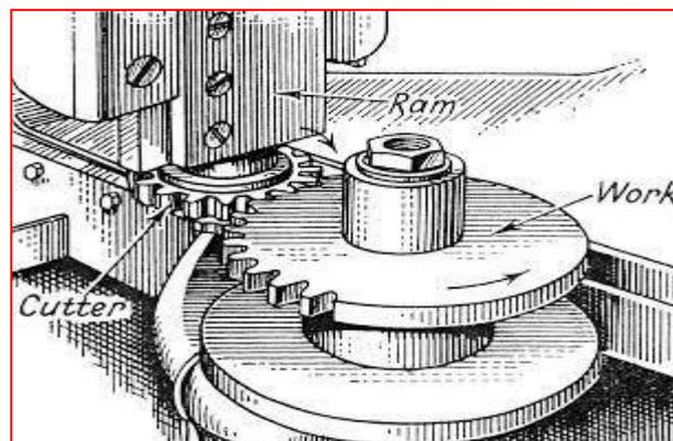
Figure 1. Principle of gear generation by rotary shaping (Boral *et al.*, 2018)
