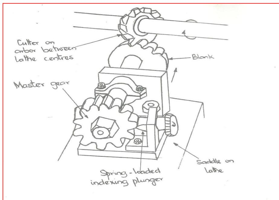
Figure 5a. Arrangement for machining spur gears on the lathe using an attachment (Amadi, 1996)
