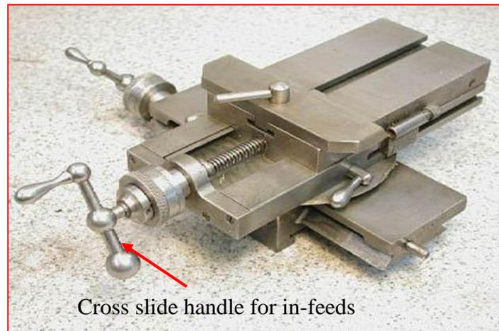
**Figure 5b. The lathe cross slide and saddle on which the spur gear machining master is attached (Amadi, 1996)**
