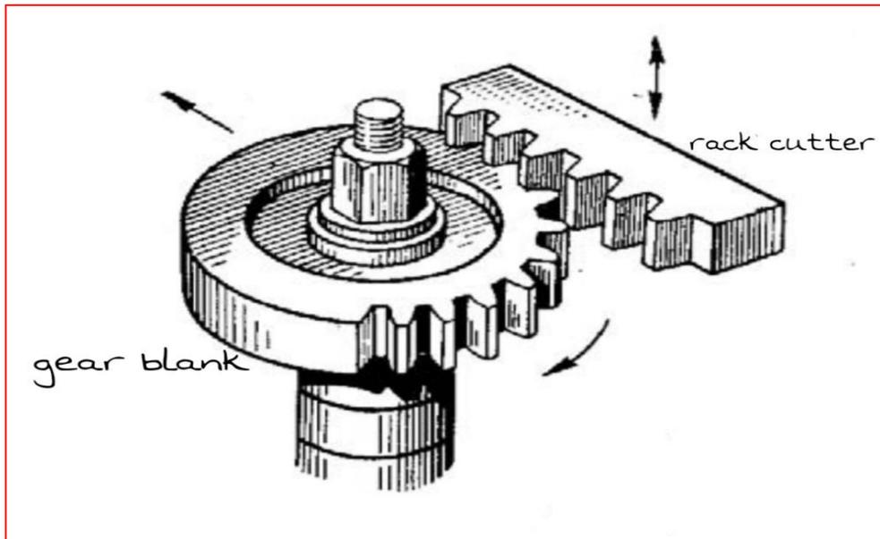
**Figure 2. Principle of gear generation by rack planning (Li *et al*, 2017)**
