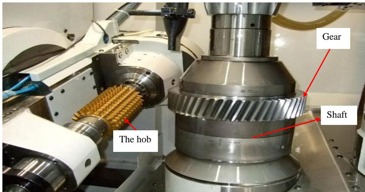
**Figure 7. Principle for hobbing spiral bevel gear (Gupta & Laubscher, 2017)**
