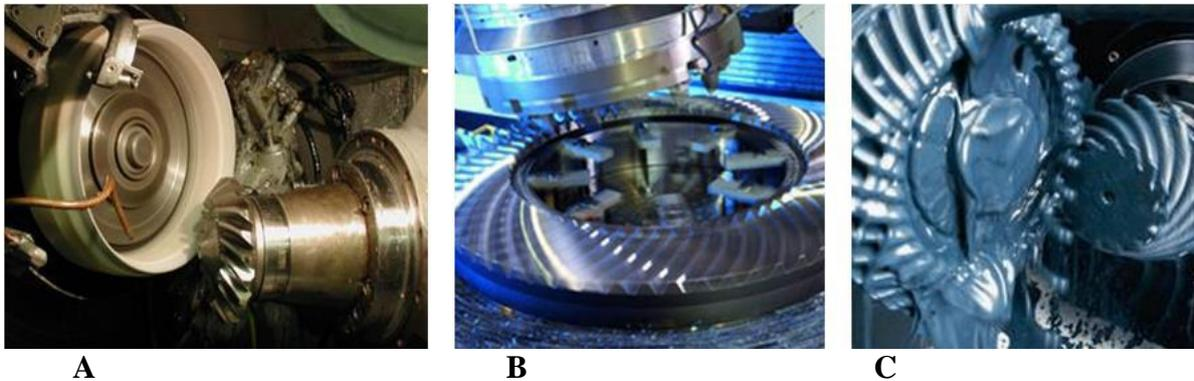
**Figure 3. (A) Gleason's gearing; (B) Cyclo-Palloid System of Klingelnberg and Oerlikon; (C) Palloid System of Klingelnberg (Kawasaki, 2010)**
