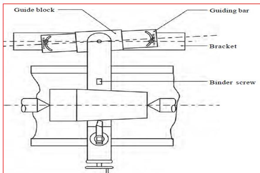
**Figure 6. A taper turning attachment for the lathe (Dalviet al, 2017)**
