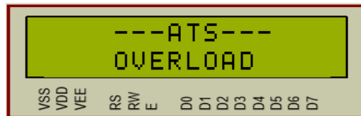
Figure 21. The LCD display showing that the system is overloaded
