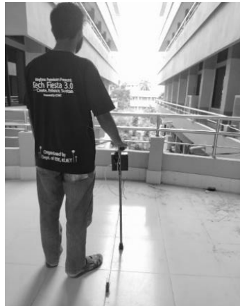
Figure 5. Experimental set up for sonar sensor in case of grid-like obstacles
