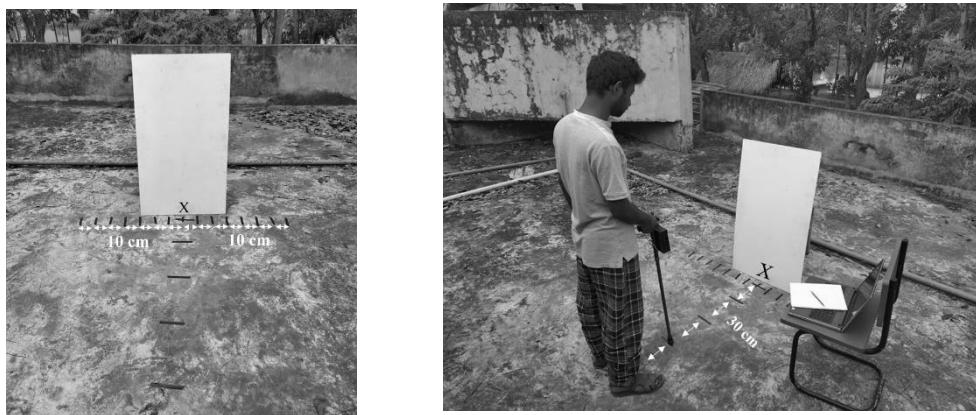
Figure 7. Experimental set up for defining workspace for sonar
