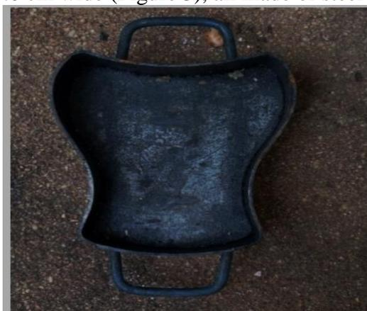
Figure 1. Sample of mold used for paving
