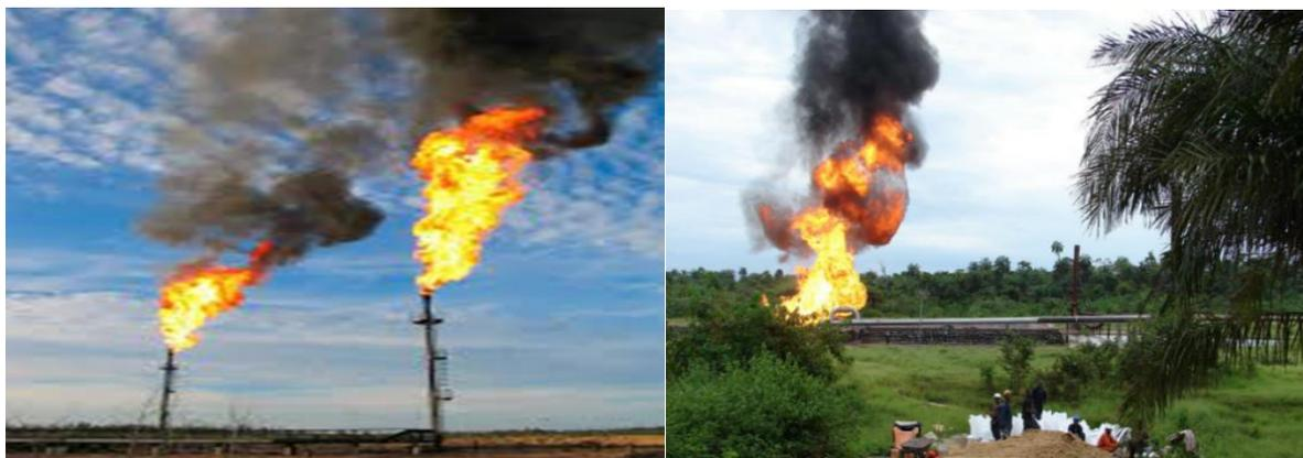
**Figure 3. Gas flaring showing emissions from turbulent diffusion flames, Niger delta**
