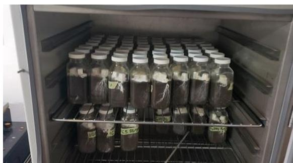
**Figure 5. Decay fungus feeding on the test specimens**
