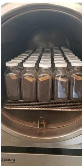
**Figure 2. Sterilization of substrate in an autoclave**
