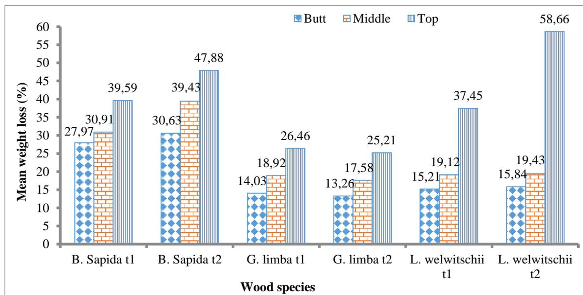
**Figure 6. Mean mass loss (%) of wood species from sections of the stem**
