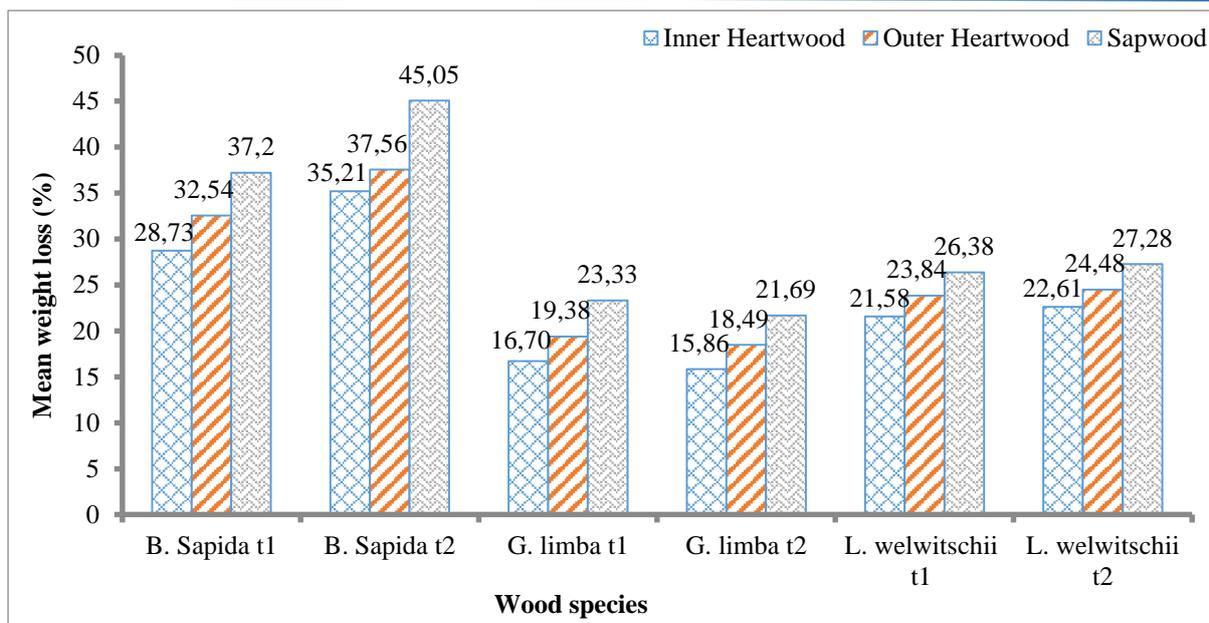
**Figure 7. Mean mass loss (%) of wood species from portions of the stems**
