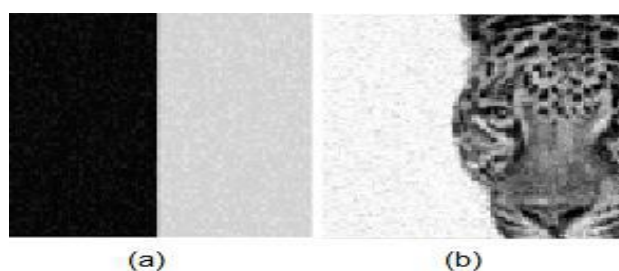
Figure 3. The effect of luminance masking HVP in (a), while the effect of texture masking HVP in (b). (Chen, 2012)
