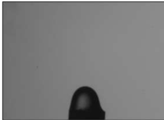
Figure 17: IFT, Low saline water mixed with surfactant at 5 cc/liter.
